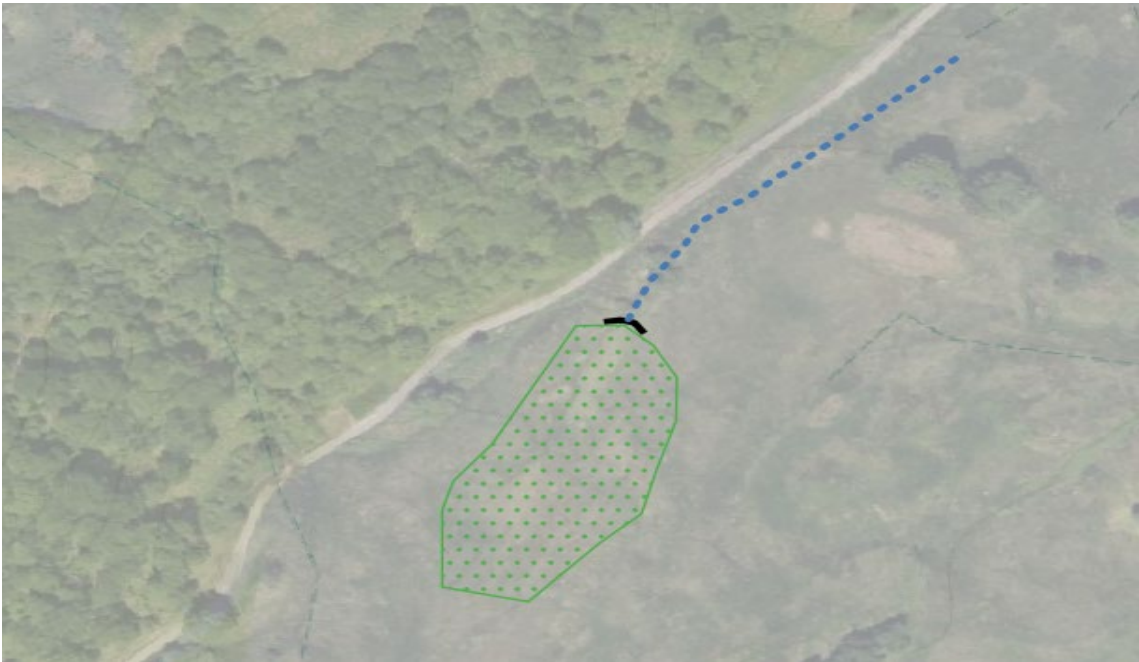
Plate 10.5.9: HMU C and area affected by drainage (green stipple) with indicative path of drainage (blue dash) and location of proposed peat bund
