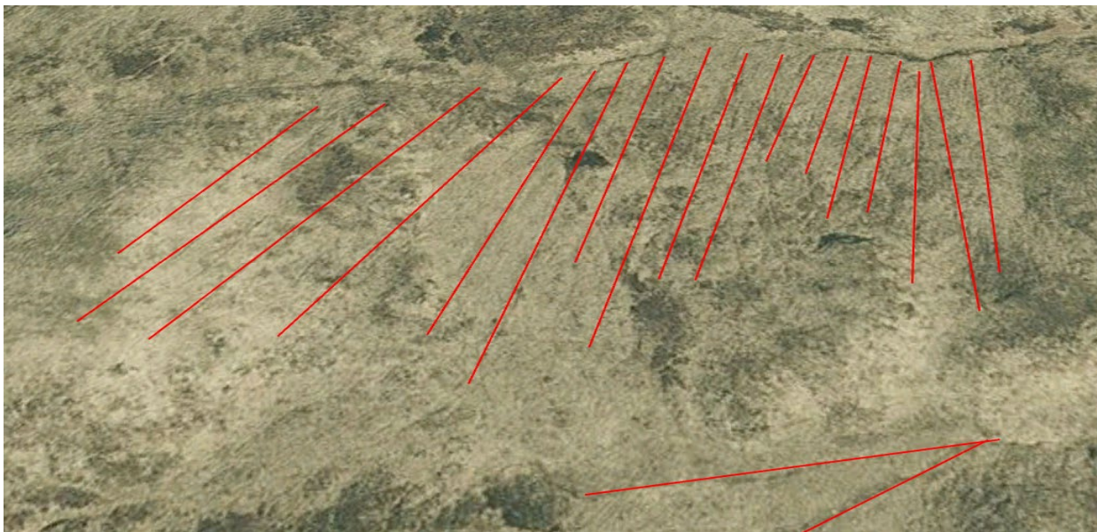
Plate 10.5.3: Example of historical on-site field drains on blanket bog (HMU A)
